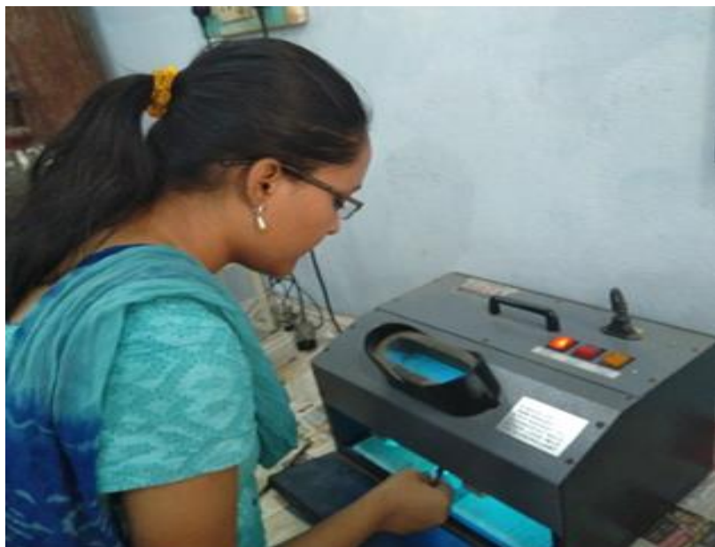
Student observing TLC under UV-detector
